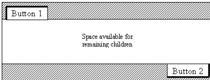
Figure 6: Adding a second button on the right side at the bottom of the layout cavity.
