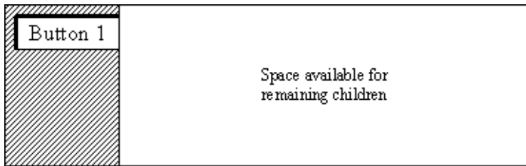
Figure 1: Creating a button on the left side and at the top of the layout cavity.
