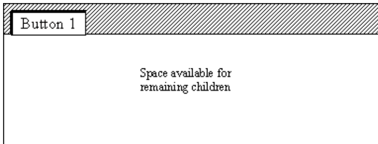
Figure 5: Creating a button on the left side and at the top of the layout cavity.
