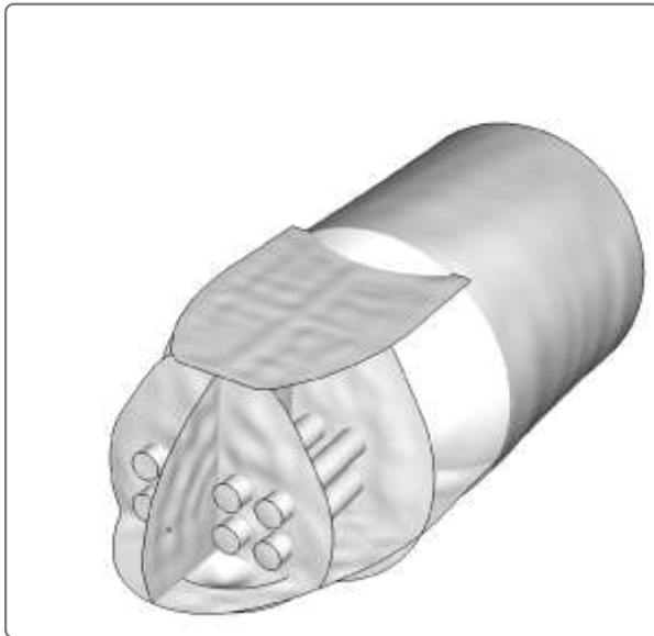
Figure 14. Deformed configuration of pressure hull, bulkheads, torpedo tubes, and sonar dome: whole view.
