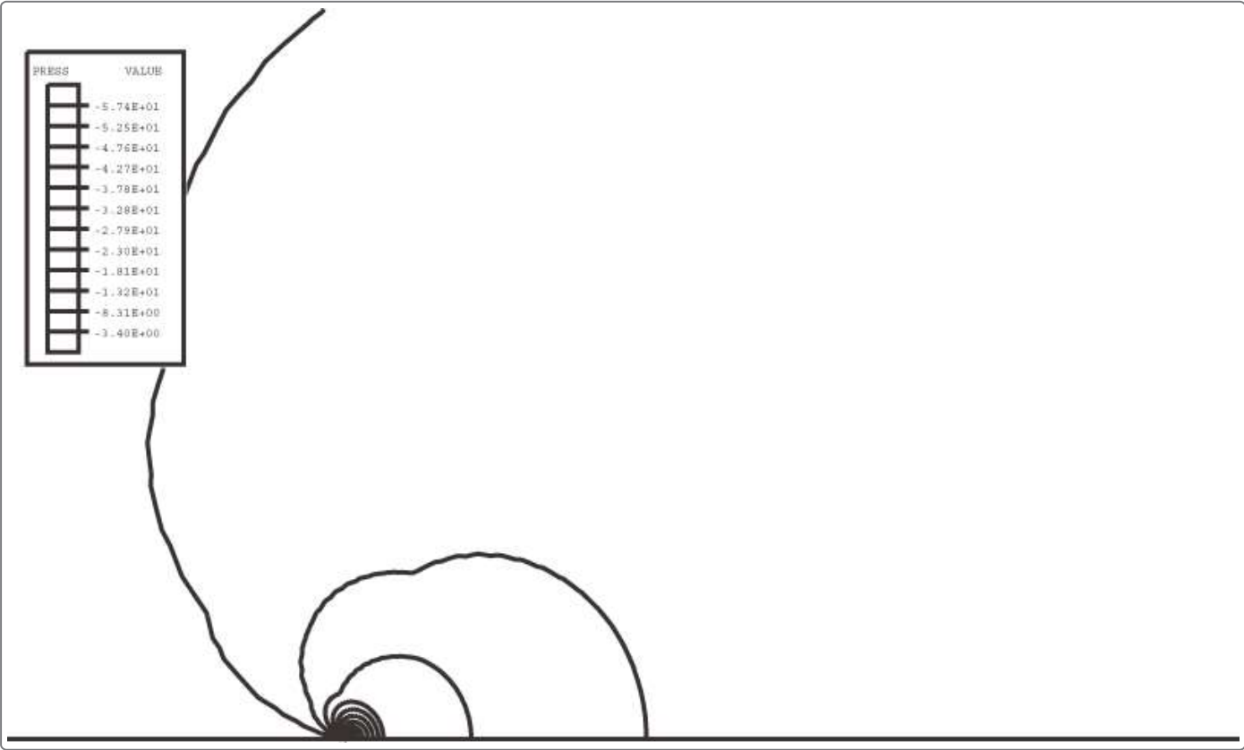
Figure 4. Contours of normalized hydrogen concentration at the crack tip.
