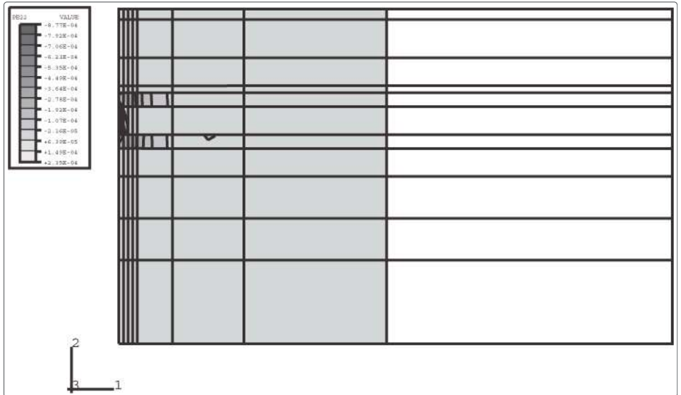
Figure 5. Contour plot of the vertical plastic strain components.
