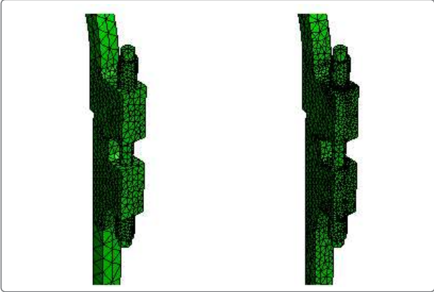
Figure 6. Original and refined mesh for the structural analysis.
