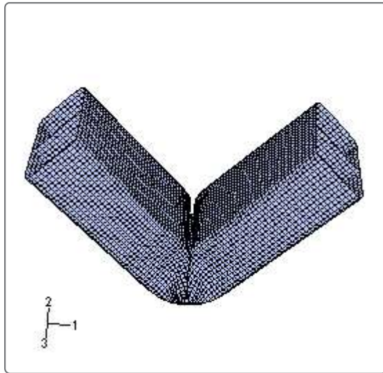
Figure 3. Deformed shape of the aluminum extrusion in the quasi-static three-point bending experiment (Hooputra et al., 2004).
