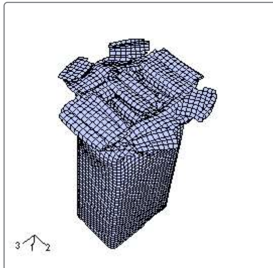
Figure 7. Final deformed shape of the aluminum extrusion in the dynamic axial crushing simulation.
