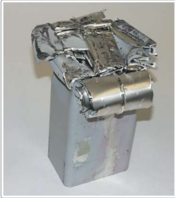
Figure 8. Deformed shape of the aluminum extrusion in the dynamic axial crushing experiment (Hooputra et al., 2004).
