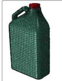
Figure 4. Tetrahedral mesh to model the fluid in the bottle in the undeformed configuration.
