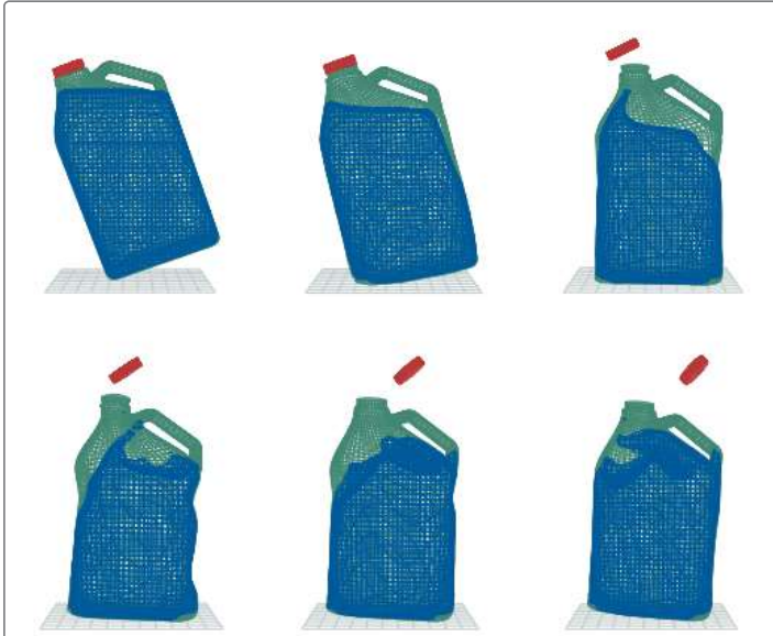
Figure 6. Logarithmic strains in the bottle during deformation in the CEL analysis.
