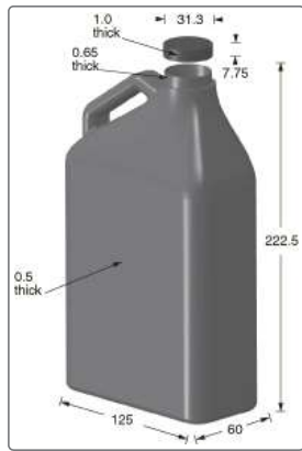
Figure 2. Assembly of the bottle drop model; the water is instanced inside of the bottle.
