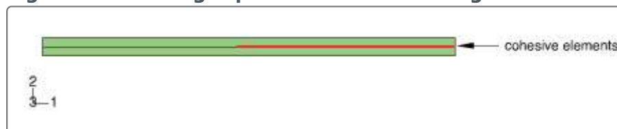
Figure 9. Modeling Z-pins and stitches using cohesive elements.
