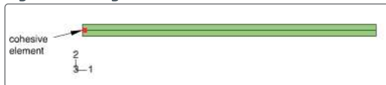
Figure 8. Using zero-thickness cohesive elements to model crack initiation.
