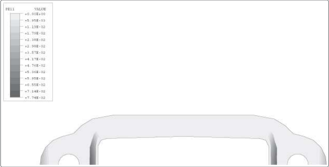
Figure 9. Plastic closure in gasket after operational cycle.
