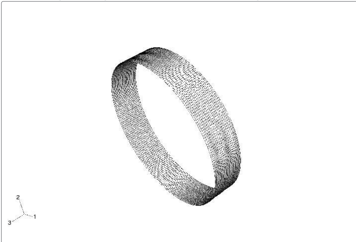
Figure 3. Perturbed geometry of the cylindrical shell (imperfection factor = 5 \times \text{thickness} for illustration only; actual imperfection factor used = .5 \times \text{thickness} ).
