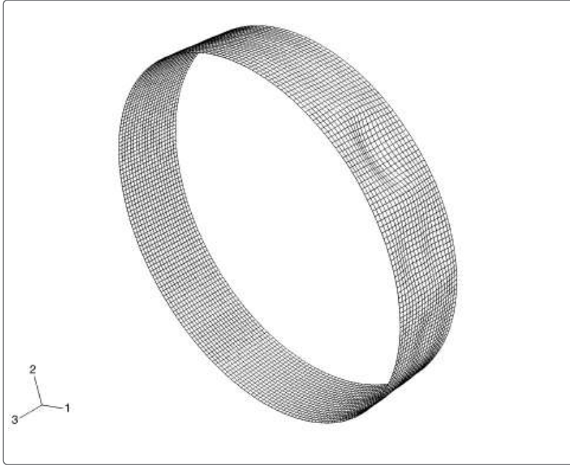
Figure 3. Perturbed geometry of the cylindrical shell (imperfection factor = 5 \times \text{thickness} for illustration only; actual imperfection factor used = .5 \times \text{thickness} ).
