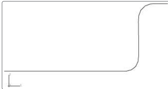
Figure 3. Deformed configuration after the first forming stage.
